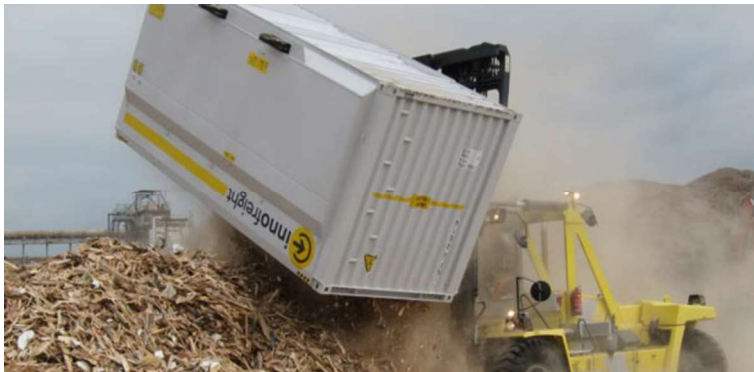
Figure 32: Unloading Innofreight containers with a forklift 78
